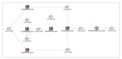
Figure 1. Juniper Secure Analytics Risk Manager topology viewer enables users to see network devices and relationships, including subnets and links.
